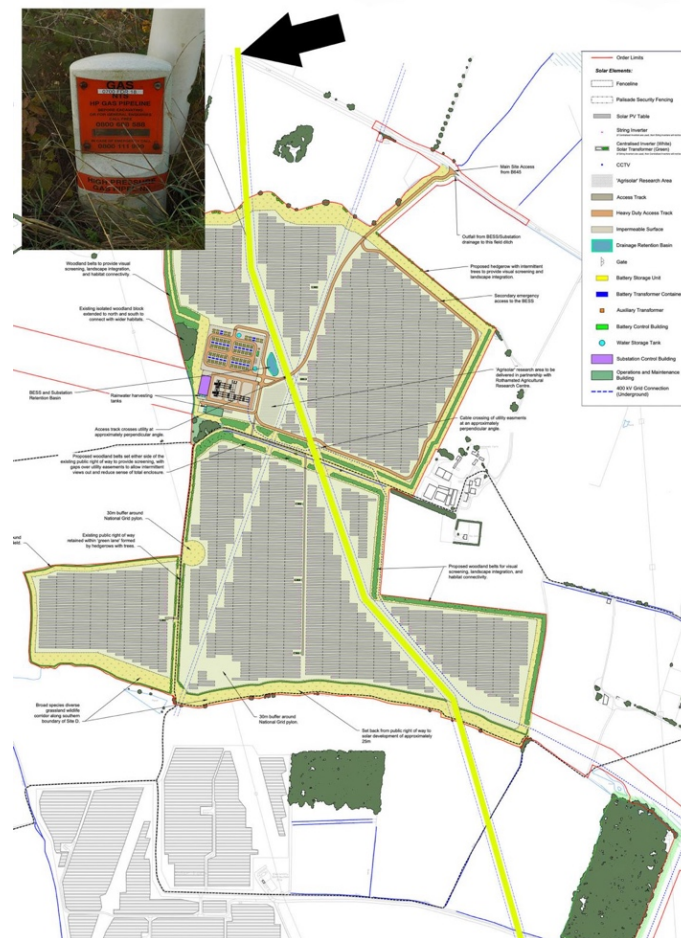
Figure 1: High-pressure gas pipeline in Site D, adjacent to BESS compound. Pipeline path marked in yellow. Arrow indicates site of Cadent high-pressure gas pipeline marker including enquiry and emergency contact details
